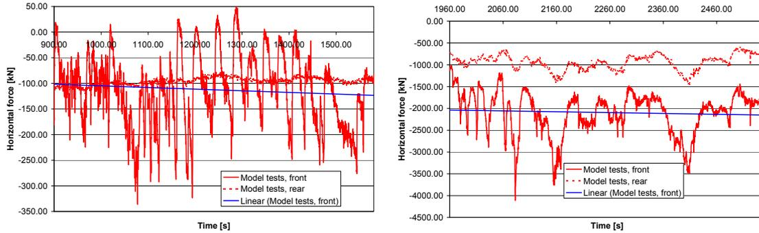
Fig. 10 Horizontal forces after a rubble pile has formed in front of the structure
