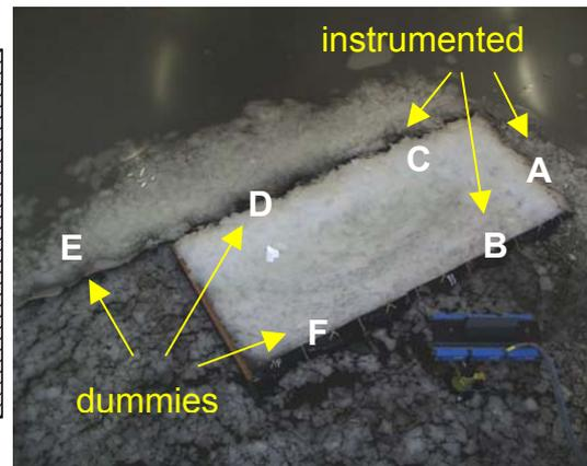
Fig. 8 'Roof type' structure filled with broken ice
