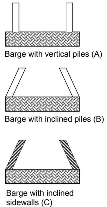
Fig. 2 Inclined ice protection piles and barges to initiate ice rubble formation
