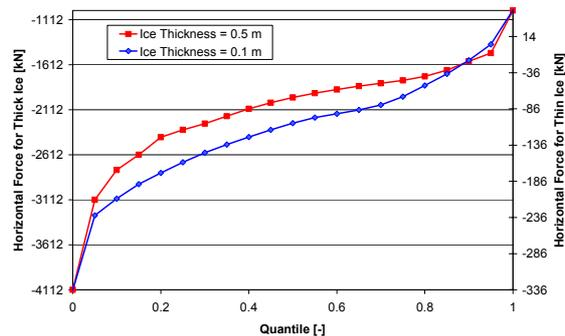
Fig. 11 Quantiles of horizontal forces for 0.1 m thick ice and for 0.5 m thick ice.
