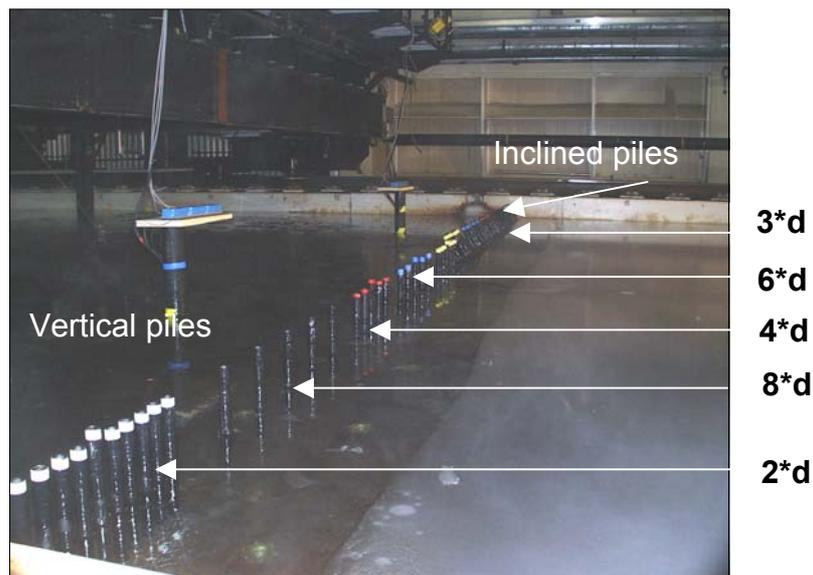
Fig. 1 Arrangement of vertical and inclined protection piles
