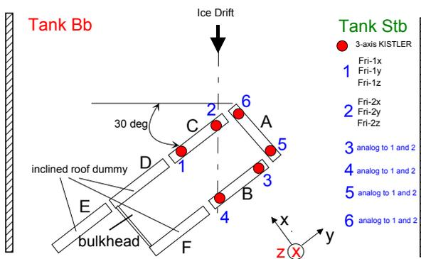
Fig. 7 Schematic of 'roof type' structure arrangement and instrumentation
