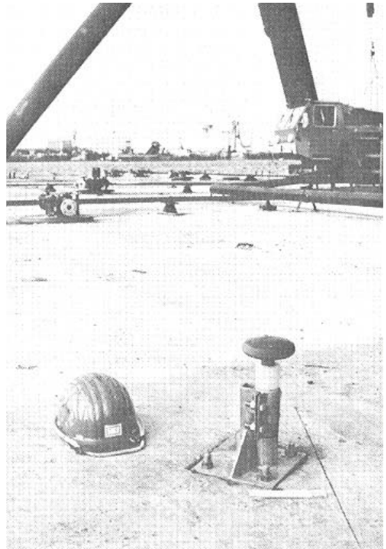
Fig. 6 Current meter on the gravity base
